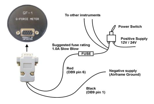
The use of an external 1A fuse is recommended. Connect the supply terminals to your aircrafts power supply. The GF-1 can be used on both 12V and 24V without the use of any pre-regulators. Ensure that the supply voltage will not drop below 8V during operation as this may result in incorrect G-force readings.
