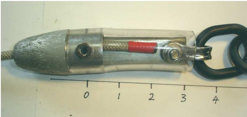
10. This shows the finished cable end piece assembly. The rope end will retract about  $\frac{1}{2}$ ” after the first tow. It is still easy to verify that the rope end has not been pulled to far in.
