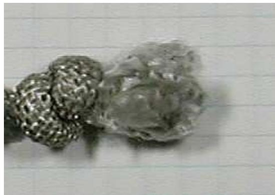
**And this is how it looks when the glider tire rolls over the rope end.**
