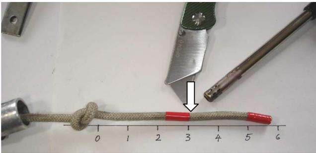
7a. Fuse the end of the rope with heat gun or flame to prevent fraying
