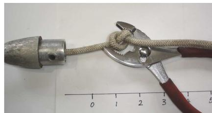
5. Apply electrical or fabric tape around rope about 3" from the knot.
