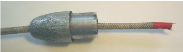
2. Push the rope end through the cable end piece.
