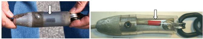
6. When the glider pilot is ready, the wing runner presents the cable end piece to him for his acceptance. Then the wing runner attaches the smaller of the Tost double rings to the glider nose tow hitch. Use proper hand signals and back your hand signals up verbally when connecting the cable end piece to the glider. The glider pilot may request a functional check of the glider tow release at this time.
