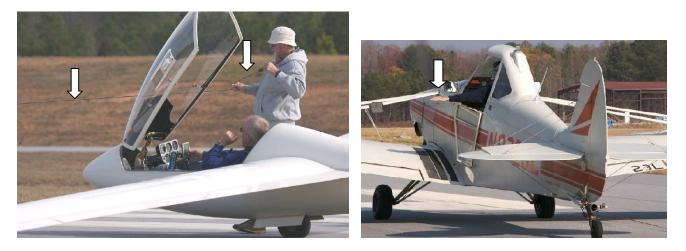
5. The wing runner should verify the taped rope end inside the clear tube of the cable end piece is visible.
