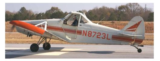
12. The tow pilot smoothly advances the throttle while holding the brakes to allow the engine to develop power (about 1500 rpm), releases the brake while continuing to add power and begins the take-off roll. This prevents a jerking motion causing the glider to roll over the tow rope, damaging the rope end.
