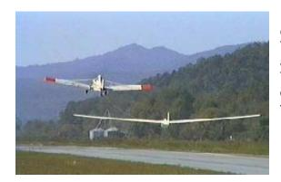
13. The tow pilot start drifting downwind of the runway centerline (20-30 deg) after reaching about 100-150 ft. This will help the glider pilot to return for landing in case of a rope break.
