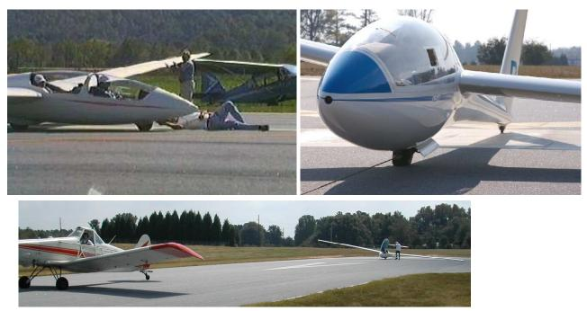
Once the tow line is attached, the wing runner moves immediately to the glider wingtip. The wing runner assures that the "Danger Zone" (the area between the glider and the tow plane) is clear and waits for the glider pilot to get ready for the launch.
