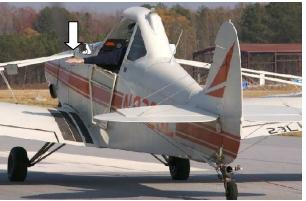
5. The wing runner should verify the red-taped rope end inside the clear tube of the cable end piece is visible.
