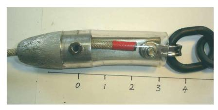
10. This shows the finished cable end piece assembly. The rope end will retract about ½" after the first tow. It is still easy to verify that the rope end has not been pulled to far in.
